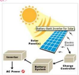
An inverter is an electrical gadget that changes over direct current (DC) to substituting current (AC); the changed over AC can be at any required voltage and recurrence with the utilization of proper transformers, exchanging, and control circuits.
